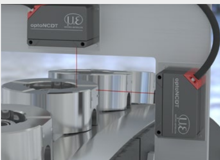
Dimension control of turned parts
