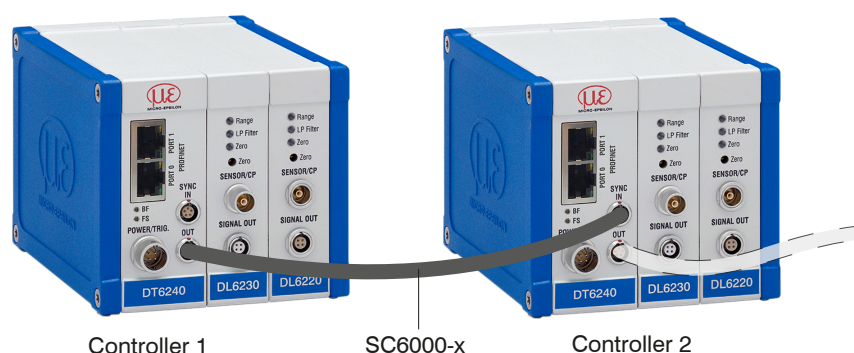
Fig. 4.14: Synchronization of a second controller
