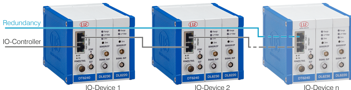
Fig. 4.15: Cabling in the PROFINET IO network
