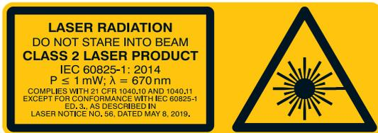
Fig. 2.1: Laser information and laser warning label
