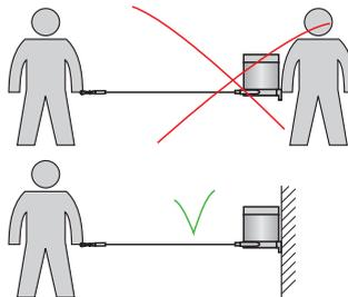
➔ Attach the measuring wire to the measured object using a wire clip.
