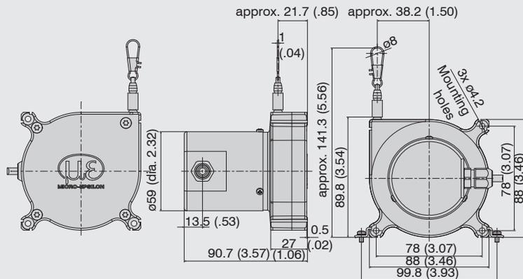
Dimensional drawing WPS-XXXX-MK88 with potentiometer, voltage, current and integrated cable, dimensions in mm (inches)
