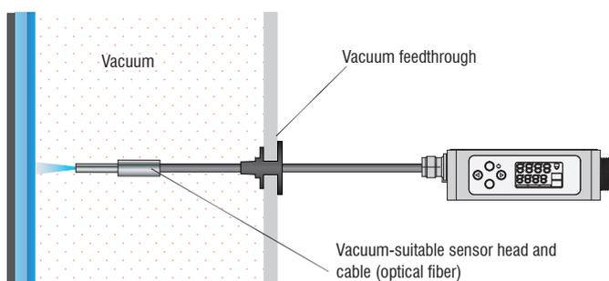
The fiber optic sensors and fiber optic cables are built with passive components and do not emit heat to the environment. In vacuum, sensors (temperature bonding T250), optical fibers (stainless steel sheath), and the vacuum feed-through up to  $10^{-5}$  mbar can be used.
