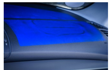
Full-surface back projection of the inspection result
